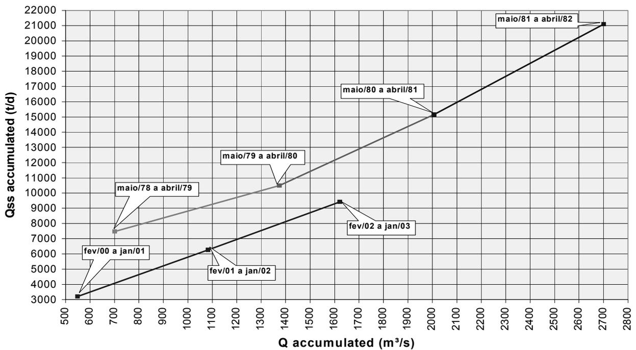
Fig. 4 Paraguay River at Cáceres, mass curve produced by plotting the accumulated river flows vs the accumulated suspended sediment fluxes.
