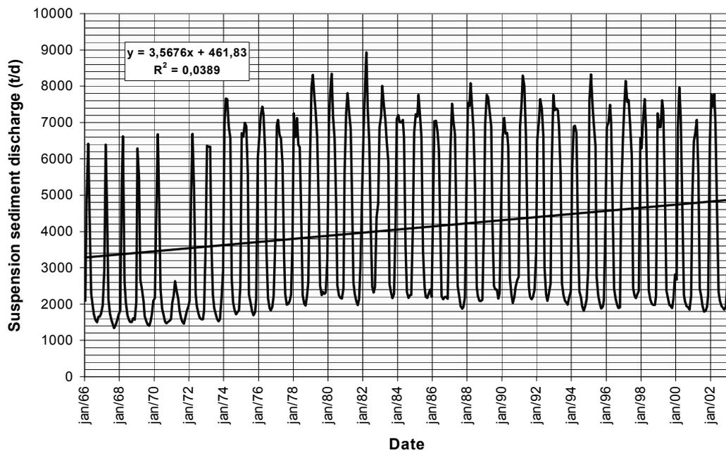
**Fig. 3** Paraguay River at Cáceres, suspended sediment discharge vs time showing an increase during the period 1966–2002.
